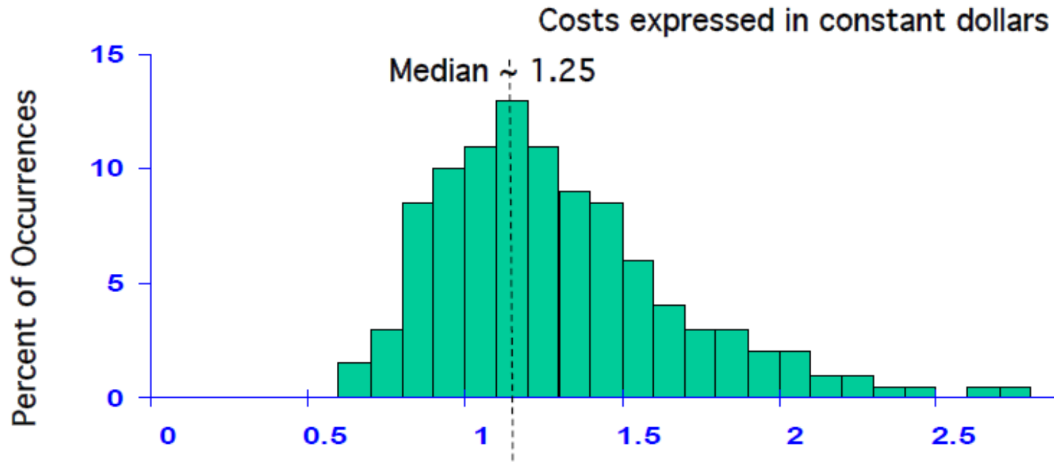
Real/Estimated Cost Ratio Repaving of runways
