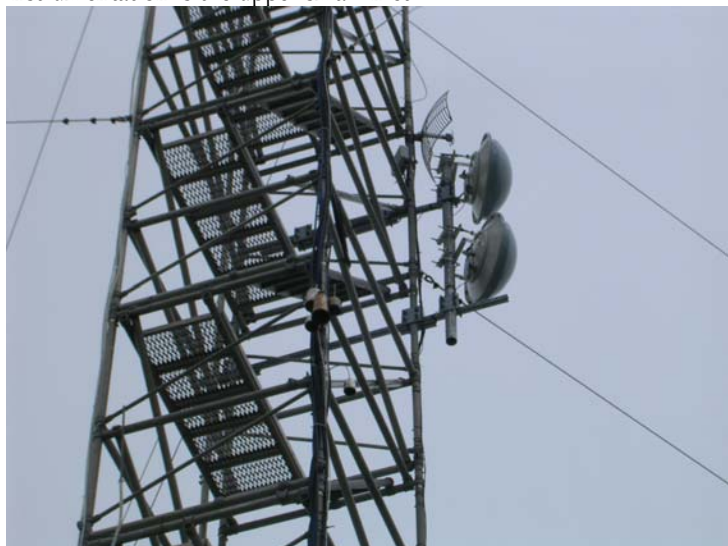
Figure A4.7 Inlets for flask sampling line and AGAGE instrumentation at 10m on the Mace Head tower.
