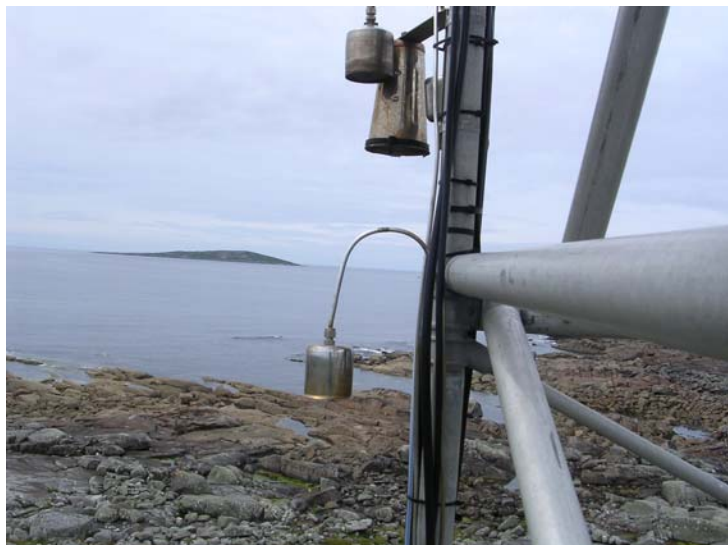
Figure A4.6 Inlets on the Mace Head tower at ~10 m. Flask sampling line is the lower small inlet, AGAGE instrumentation is the upper small inlet.
