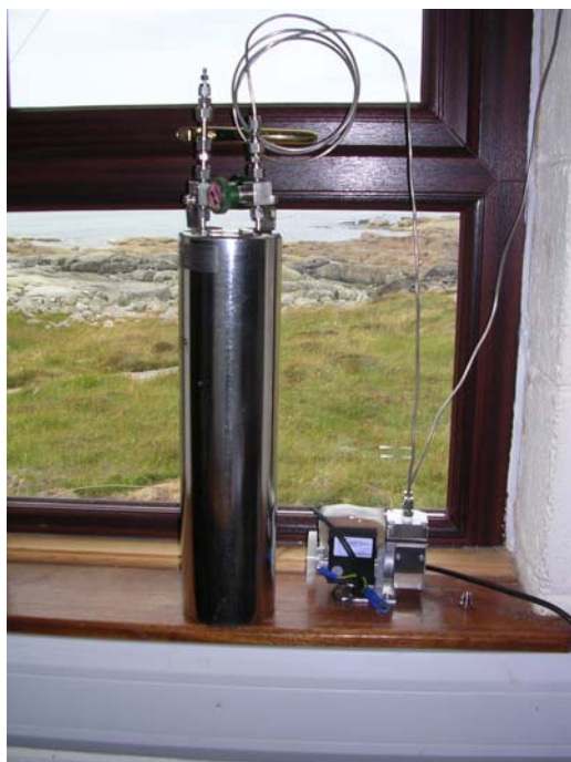
Figure A4.5. Air sampling setup with double inlet flask. Stainless steel inlet line is connected to a Viton-free diaphragm pump which is used to flush and then fill the flask to ~3-4 bar a through the dip-tube inlet.
