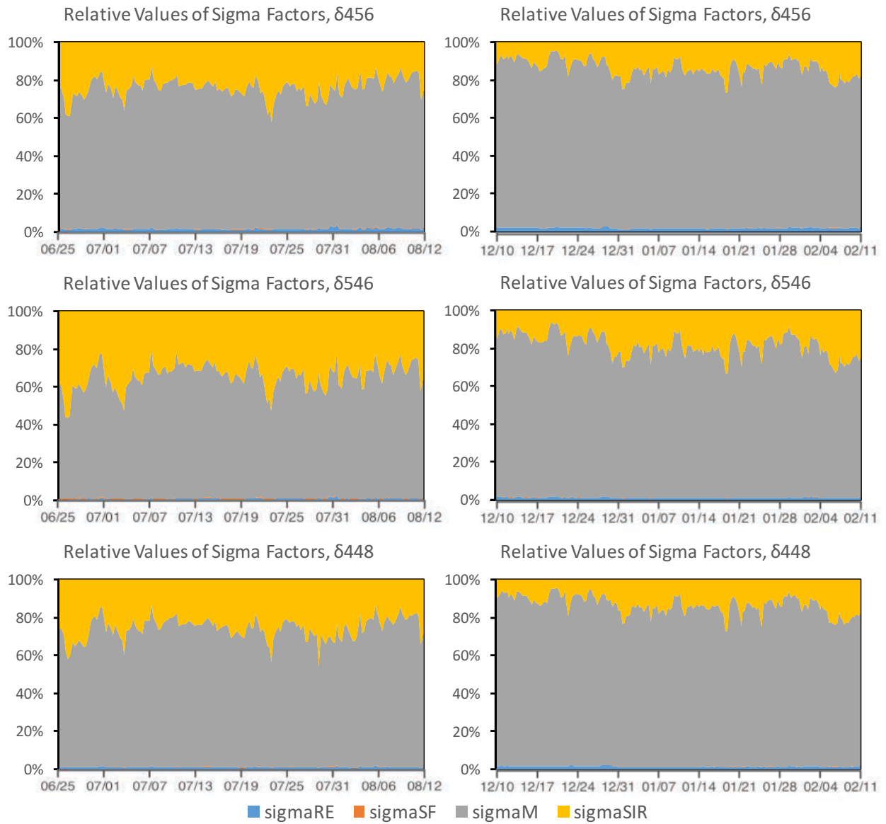
Figure 6-19: Relative contribution to \sigma^2 from the four factors \sigma_M , \sigma_{RE} , \sigma_{SF} , and \sigma_{SIR} for the three N_2O isotopic ratios
