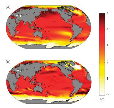
**Figure 2.** (a) Ensemble-average SST anomalies 100 years after an abrupt quadrupling of  $CO_2$  in 15 CMIP5 models. (b) SST anomalies after 100 years of an ocean only configuration of the MITgcm induced by a uniform downwelling flux of 4 W m<sup>-2</sup> and damped at a uniform rate of 1 W m<sup>-2</sup> K<sup>-1</sup>, as described in §2.
